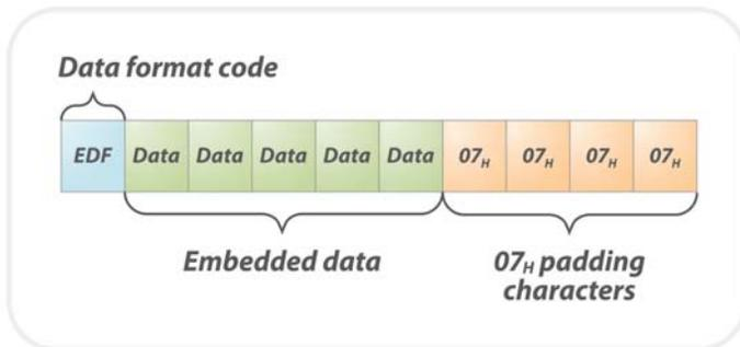
Figure 4: MIPI CCS Embedded Data Line Format
