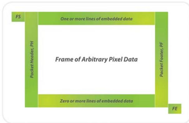
Figure 3: MIPI CCS Use of Embedded Data to Sync Host and Sensor
