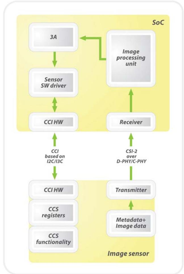
Figure 1: Typical Camera System with CCS
